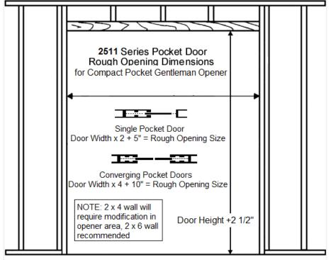
Example: 30" (Door size) x 2 = 60" + 5"(needed for opener) = 65" Rough Opening
